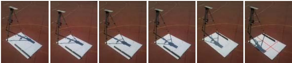
Figure 12. Procedure for calculating the true noon
