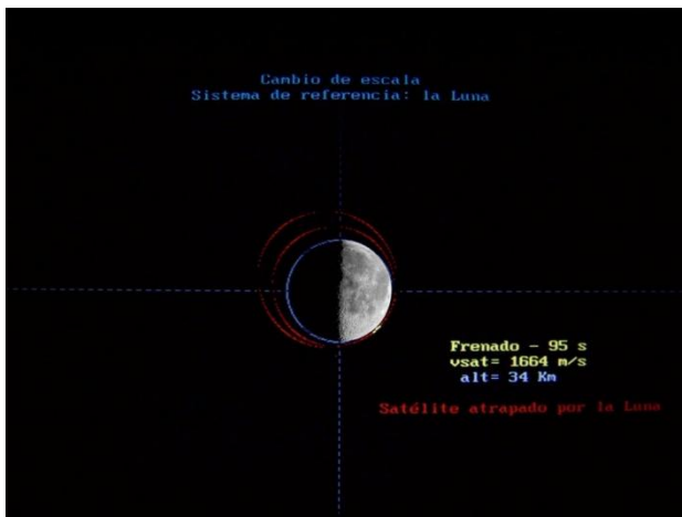
Figures 17 y 18: Two brakes to low circular orbit
